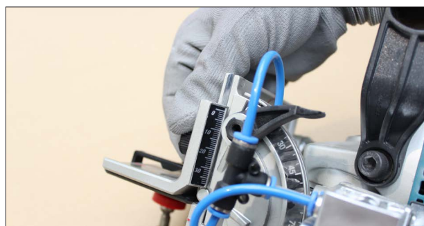
4. Adjust tool based on final position of kerf and thickness of panel.
