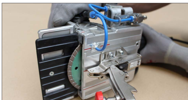
3. Check blade is in good condition.
