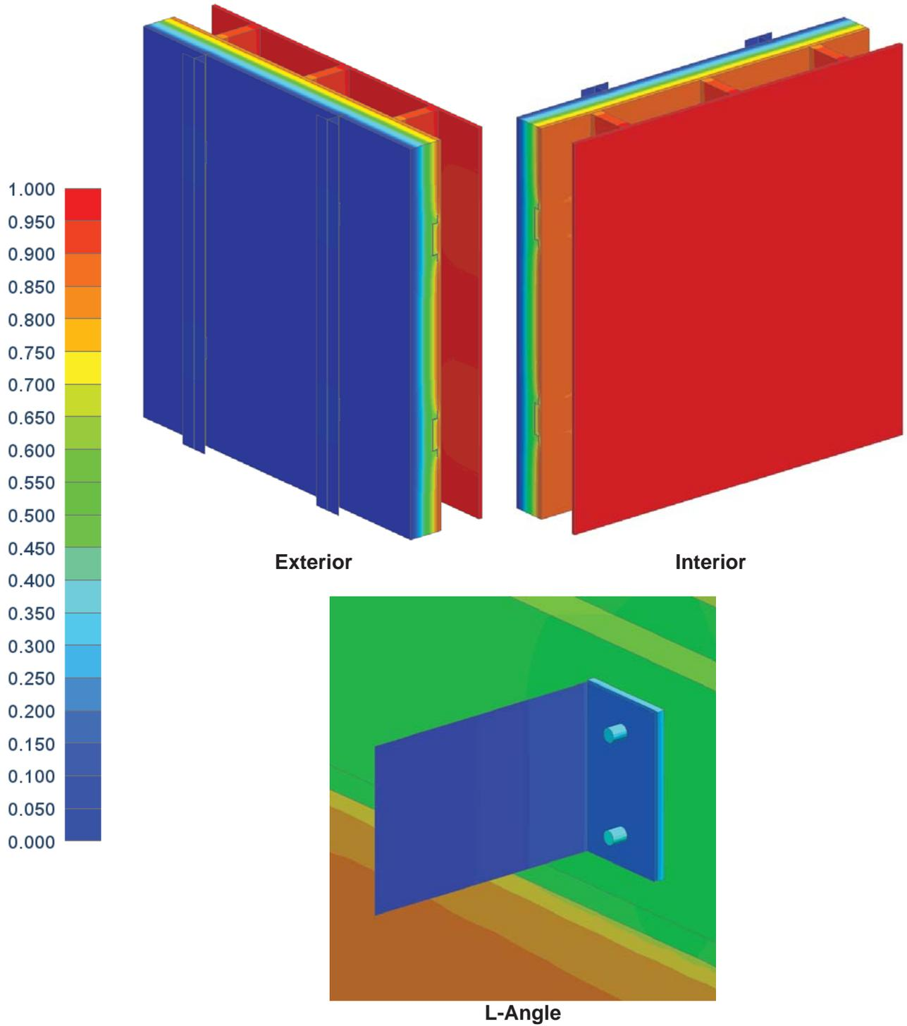
Figure C6: Split Insulated Wood Framed Wall with Omega Bar
