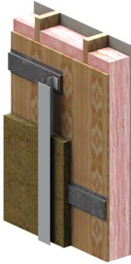
The thermal transmittance U-value results of the Porcelanosa Cladding Attachment System with a split insulated wood framed wall are presented in Table 3.6.
