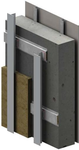
The thermal transmittance U-value results of the Porcelanosa Cladding Attachment System and Omega Bar with a concrete mass wall are presented in Table 3.2.
