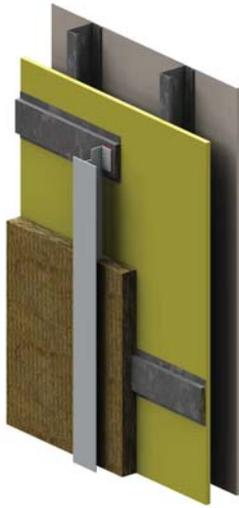
The thermal transmittance U-value results of the Porcelanosa Cladding Attachment System and Omega Bar with an exterior insulated steel stud wall are presented in Table 3.3.
