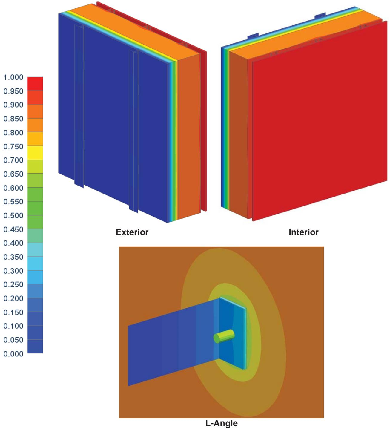
Figure C2: Exterior Insulated Concrete Mass Wall with Omega Bar
