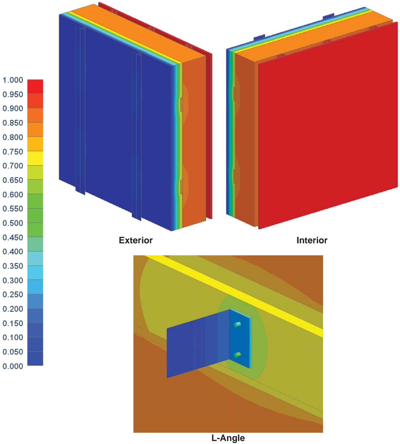
Figure C3: Exterior Insulated Steel Stud Wall with Omega Bar
