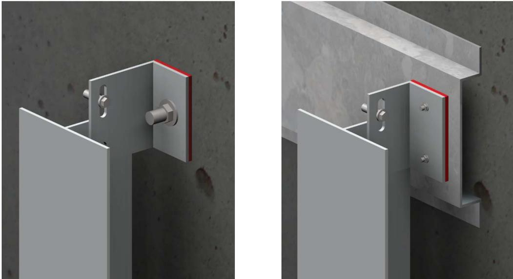
Figure1.1: Simplified Rendering of Porcelanosa Cladding Attachment
