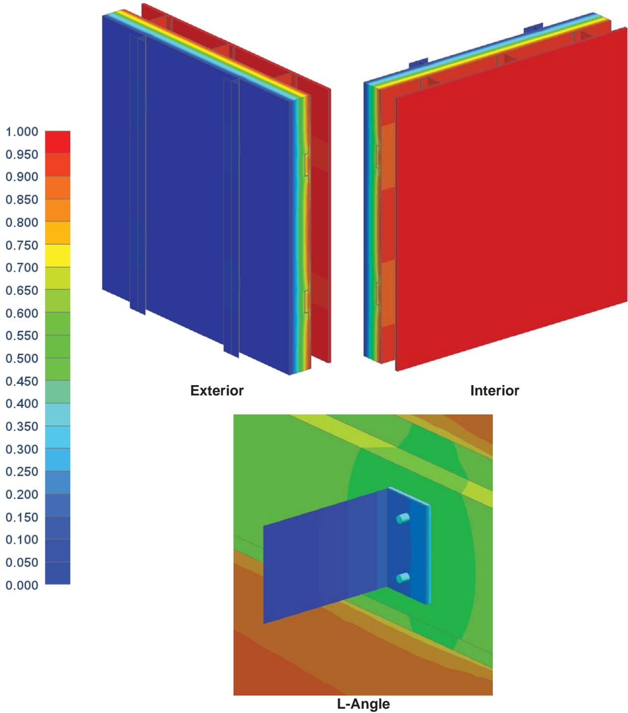
Figure C4: Split Insulated Steel Stud Wall with Omega Bar
