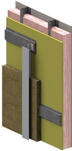
The thermal transmittance U-value results of the Porcelanosa Cladding Attachment System and Omega Bar with a split insulated steel stud wall are presented in Table 3.4.
