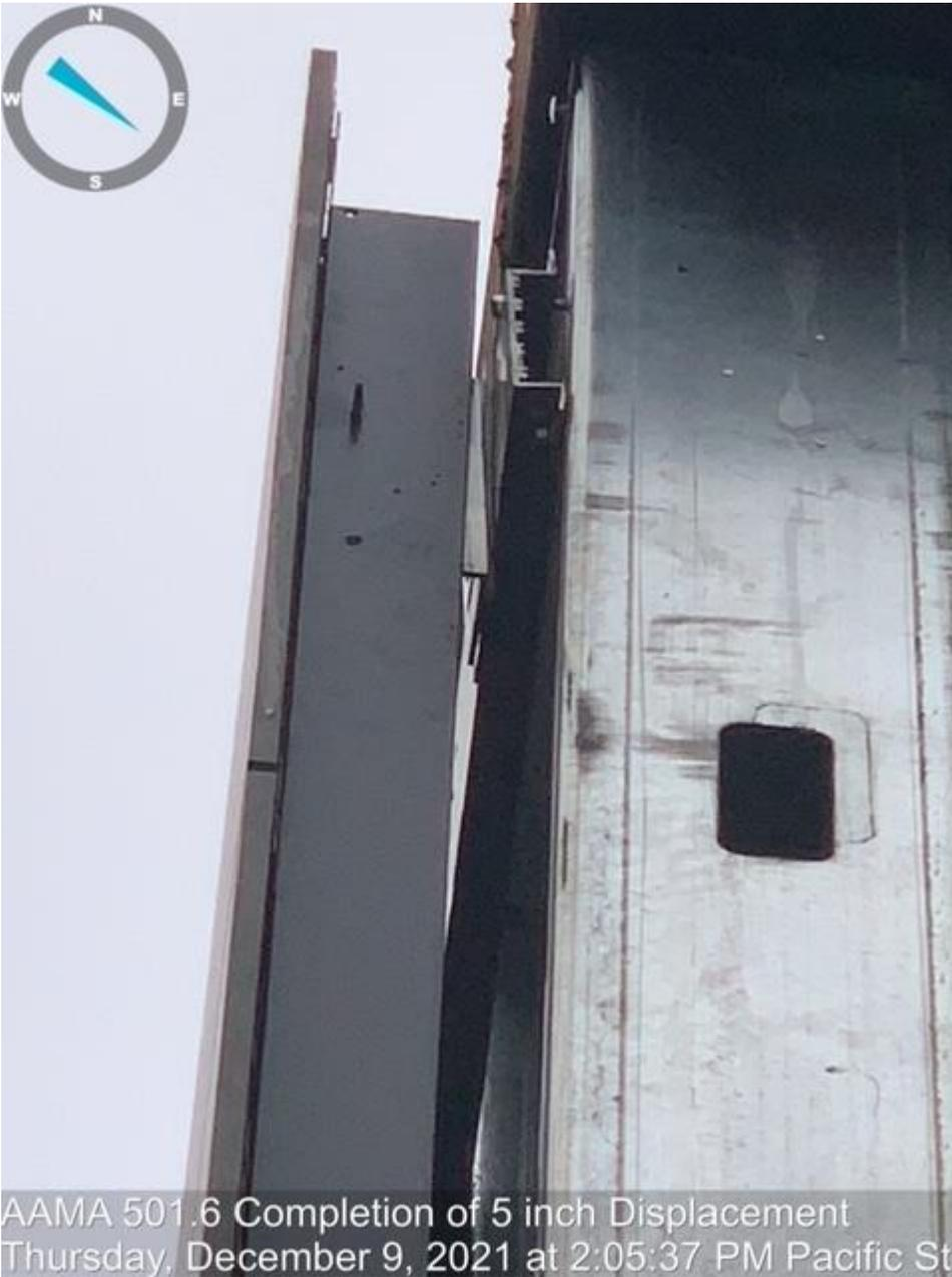
AAMA 501.6 Completion of 5 inch Displacement
