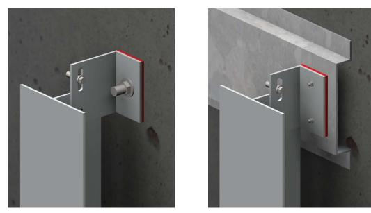
Figure 1.1: Simplified Rendering of Porcelanosa Cladding Attachment
