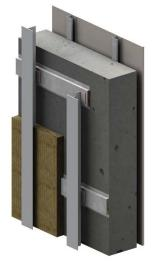
**Figure 3.3**: Concrete Configuration with Omega
