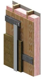
Figure 3.7: Split Insulated Wood Frame Configuration
