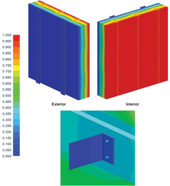
Figure C4: Split Insulated Steel Stud Wall with Omega Bar
