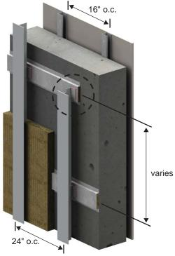
Exterior Insulated Concrete Mass Wall with Omega Bar Hat Channel
