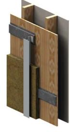
**Figure 3.6**: Exterior Insulated Wood Frame Configuration
