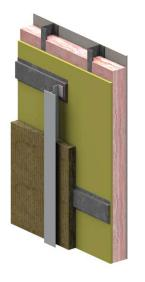
Figure 3.5: Split Insulated Steel Frame Configuration with Omega
