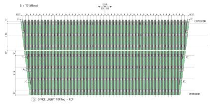
Soffit substructure layout shop drawing example.
