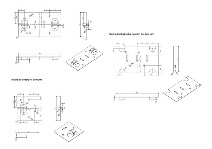
FIGURE 2—STAINLESS STEEL FIXING CLIPS
