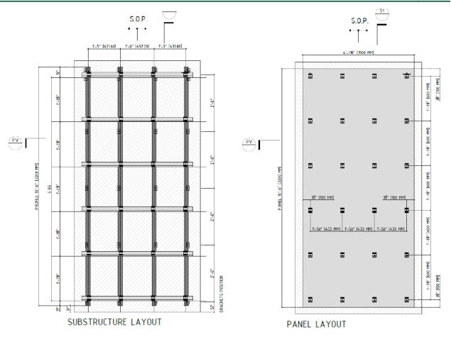
FIGURE 3 - XTONE SUBSTRUCTURE AND PANEL LAYOUT
